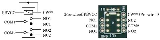
For mechanical relay signals, paired GND to relay pins do not exist.
